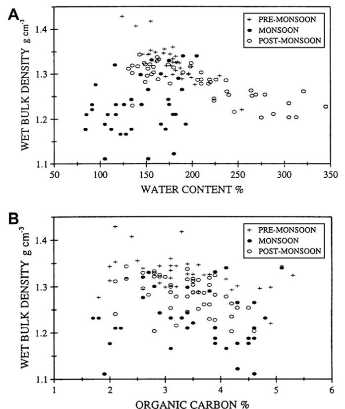
Fig. 8. Bivariate plots of (A) water content versus wet bulk density, and (B) organic carbon content versus wet bulk density.
