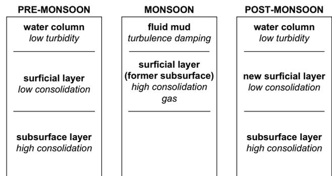
Fig. 7. Schematic of sediment dynamic processes in the mudbank during different seasons. Pre-monsoon: low SSC water column overlying seabed sediment that becomes more consolidated with depth. Monsoon: erosion of surficial layer exposes more consolidated subsurface layer and generates benthic fluid mud and high SSC in water column. Post-monsoon: fluid mud and re-suspended sediment settle back to bed as a low consolidation layer and SSC declines.
