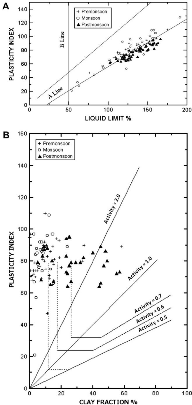
Fig. 6. Atterberg limits of mudbank sediments: (A) plasticity chart, and (B) activity chart.
